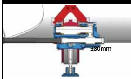
Figure 8: Bogiflex KGD radial movement capacity
