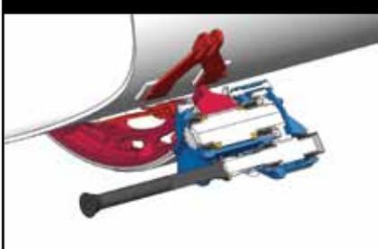
Figure 7: Bogiflex KGD axial and tilting movement capacity
